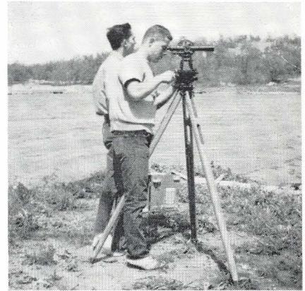
Students are checking survey instruments used in determining surface area and establishing depth contours on a field exercise.
