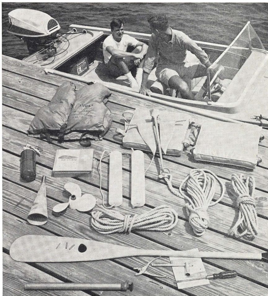
Choosing the proper equipment for both fun and safety will make your boating more enjoyable. The equipment shown here includes Coast Guard approved life jackets and cushions, anchor with plenty of line, fire extinguisher, first-aid kit, horn, extra propeller, fenders and extra line. On the paddle are extra cotter pins, drive pins and propeller nut. At the bottom is a bilge pump, basic tools and an outboard owner's manual.
